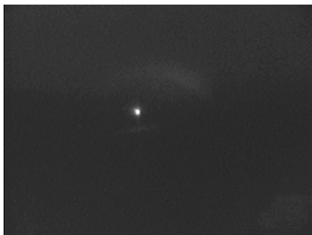
Fig. 10. Near-field mode pattern for TE polarized light at 1550 nm.
